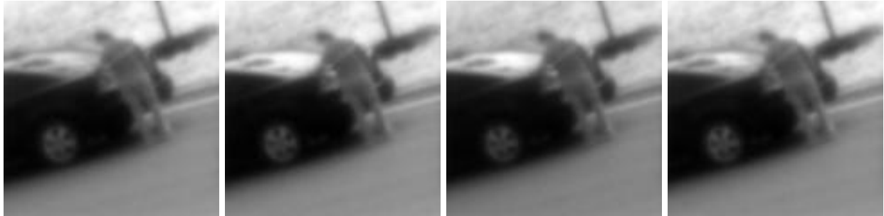
Figure 1. Noisy and blurred polarimetric imagery. From left to right the angle of the polarizer is \{0^\circ, 45^\circ, 90^\circ, 135^\circ\}
