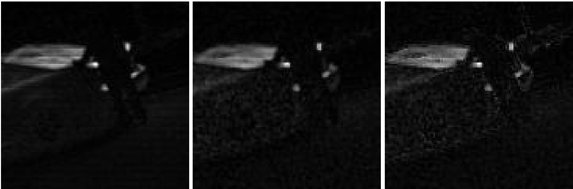
Figure 6. Estimates of DOLP. From left to right: Pristine, Proposed Method, Traditional Method
