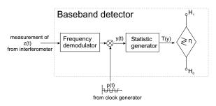
Fig. 3. Baseband detector frequency demodulates the interferometric signal, correlates the output against a square wave p(t) whose transitions are synchronous with the turn-off times of the RF field  $\mathbf{B}_1(t)$ , and generates a test statistic, for detecting presence of a spin.
