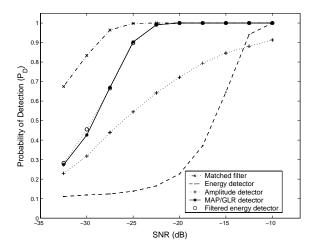
Fig. 5. Power curves ( $P_{\rm D}$  vs. SNR) for the five detectors considered in this paper for  $P_{\rm F}=0.1$  and  $\lambda=1$  per-second. At  $P_{\rm D}=0.8$  both the hybrid Bayes/GLR and filtered energy detector performed within 4 dB of the bound established by the matched filter.
