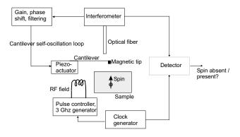
Fig. 1. Schematic of the OSCAR experiment.
