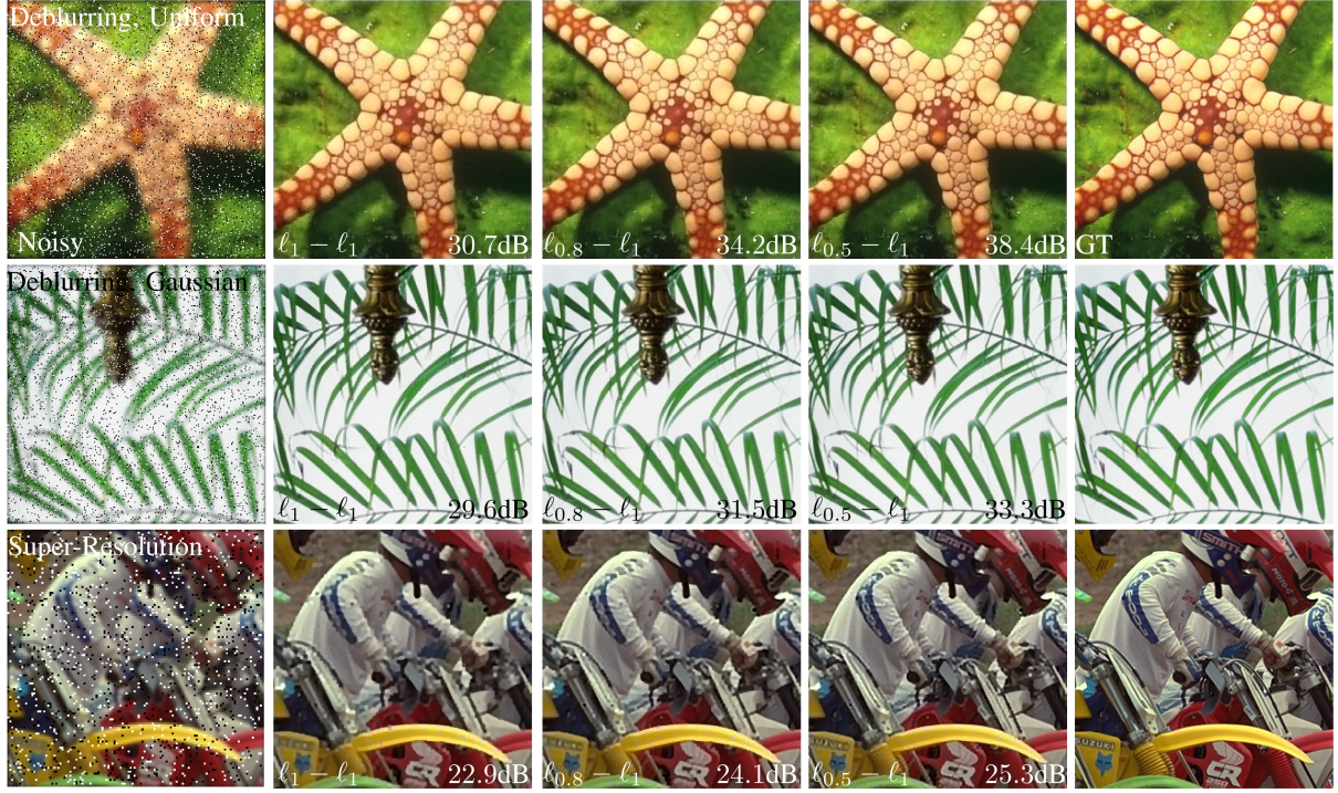
Fig. 3. The reconstructed images for different p on the image deblurring (first and second rows) and super-resolution (third row) tasks. The PSNR value is labeled at the right bottom corner of each image. The first and fifth columns are the noisy measurement and the ground truth, respectively. The first (respectively, second) row is the reconstructed starfish (respectively, leaves) image at 10th (respectively, 6th) iteration for the image deblurring task with uniform (respectively, Gaussian) blur. The third row is the reconstructed bike image at 7th iteration for the image super-resolution task with a downsampling factor 2 and 5% salt-and-pepper noise.
