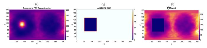
Fig. 3. (a) First iteration of LM-MLEM of the background FOV which is multiplied by the (b) apodizing  $\cos^2$  mask that smoothly transitions to the ROI where all pixel values go to zero in the (c) masked background projection.
