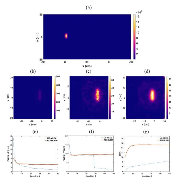
Fig. 5. 22nd iteration reconstructions of a simulated 10 cm  $^{137}$ Cs line source in a (a)  $4\pi$  LM-MLEM reconstruction, (b) LM-MLEM in a 90° FOV, (c) LM-MLEM 90° FOV with the outermost 10 edge pixels removed, and (d) ROI-MLEM reconstruction in a 90°. (e) and (f) Compares the FWHM values in the *x*- and *y*-directions, respectively, for both imaging algorithms, and (g) compares the SNR values for 50 iterations of both methods.
