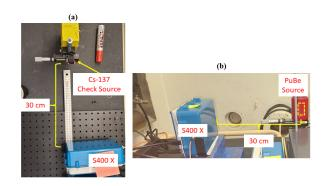
Fig. 4. (a) <sup>137</sup>Cs experimental setup, the micrometer is used to shift the source from the "no shift" measurement location to the right by 3, 5, and 10 mm, each for 1-h measurements. (b) PuBe source experimental setup, the PuBe peg is an extended source approximately 2 in in length and 1 in diameter placed inside a small lead container 30 cm away from a S400X system. The source is shifted from left to right by 1 cm for two separate 3-h measurements.
