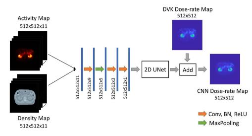
FIGURE 3 The architecture of our DblurDoseNet
