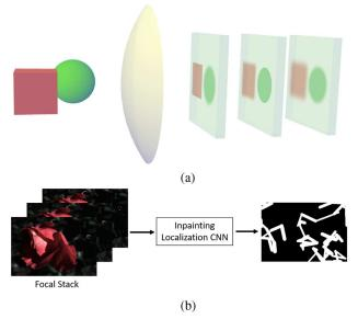
**Fig. 1.** Focal stack system for inpainting region localization. (a) Imaging system schematic showing depth-dependent defocus blur of a cube-ball object. (b) Inpainting localization CNN estimates inpainting regions from a focal stack.
