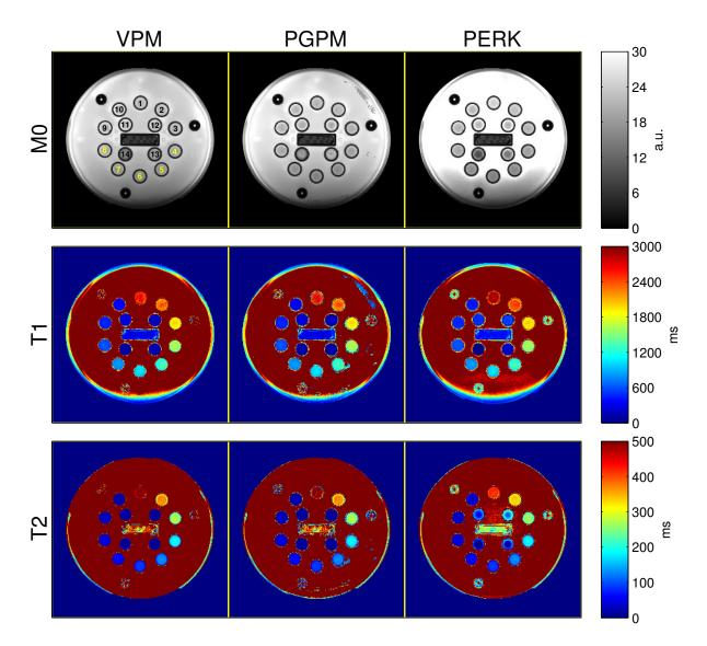
Figure S.7: VPM, PGPM, and PERK  $M_0$ ,  $T_1$ ,  $T_2$  estimates in a quantitative phantom. Vials are enumerated and highlighted to correspond with markers and colored boxes in Fig. 1. PERK has only been trained to accurately estimate within vials 4-8; within these vials, VPM, PGPM, and PERK estimates appear visually similar.
