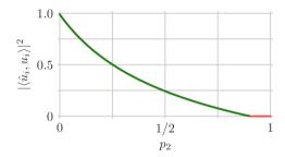
**Fig. 2.** Asymptotic subspace recovery (4) of the *i*th component as a function of the contamination fraction  $p_2$ , the proportion of samples with noise variance  $\sigma_2^2 = 3.25$ , where the other noise variance  $\sigma_1^2 = 0.1$  occurs in proportion  $p_1 = 1 - p_2$ . The sample-to-dimension ratio is c = 10 and the subspace amplitude is  $\theta_i = 1$ . The region where  $A(\beta_i) \le 0$  is the red horizontal segment with value zero (the prediction of Conjecture 1).
