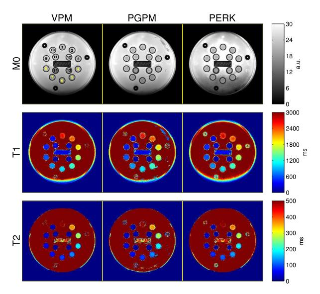
Figure S.9: More aggressively trained VPM, PGPM, and PERK  $M_0, T_1, T_2$  estimates in a quantitative phantom. Here the PERK estimator was trained with a sampling distribution whose support extended over less well identified  $T_1, T_2$  values. Comparing with analogous images in Fig. S.7, PERK performance within vials 4-8 degrades, though in other vials performance clearly improves. Vials are enumerated and highlighted to correspond with markers and colored boxes in Fig. S.8.
