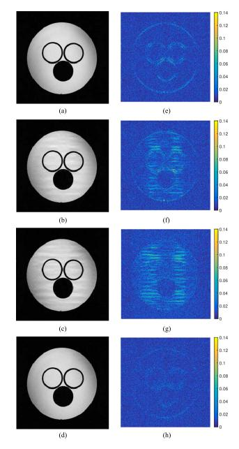
Fig. 6. Results for Image (c) with Cartesian sampling and 2.5x undersampling. The sampling mask is shown in Fig. 5(a). Reconstructions (magnitudes): (a) DLMRI [13]; (b) PANO [75]; (c)  $\ell_0$  "norm"-based FDLCP [18]; and (d) SOUP-DILLO MRI (with zero-filling initialization). (e)-(h) are the reconstruction error maps for (a)-(d), respectively.
