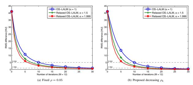
Fig. 2: XCAT: Convergence rate curves of relaxed OS-LALM (12 subsets) using different values of the over-relaxation parameter  $\alpha$  with (a) fixed AL penalty parameter  $\rho = 0.05$  and (b) proposed decreasing  $\rho_k$ .
