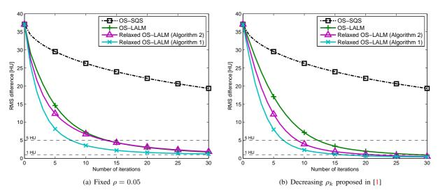
Fig. 7: Chest: Convergence rate curves of different relaxed algorithms (10 subsets and  $\alpha = 1.999$ ) with (a) a fixed AL penalty parameter  $\rho = 0.05$  and (b) the decreasing sequence  $\rho_k$  proposed in [1].
