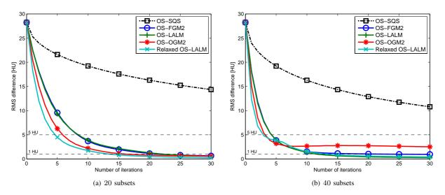
Fig. 11: Shoulder: Convergence rate curves of different OS algorithms with (a) 20 subsets and (b) 40 subsets. The proposed relaxed OS-LALM with 20 subsets exhibits similar convergence rate as the unrelaxed OS-LALM with 40 subsets.
