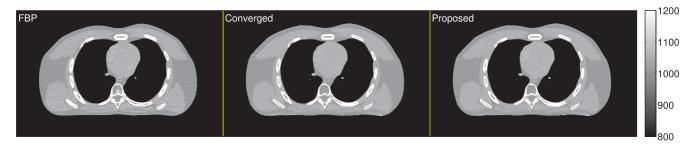
Fig. 1. XCAT: Cropped images (displayed from 800 to 1200 HU) from the central transaxial plane of the initial FBP image  $\mathbf{x}^{(0)}$  (left), the reference reconstruction  $\mathbf{x}^*$  (center), and the reconstructed image  $\mathbf{x}^{(20)}$  using the proposed algorithm (relaxed OS-LALM with 12 subsets) after 20 iterations (right).
