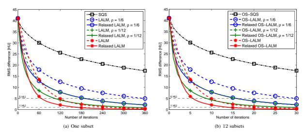
Fig. 5: XCAT: Convergence rate curves of unrelaxed/relaxed OS-LALM using different parameter settings with (a) one subset and (b) 12 subsets. All algorithms run 360 subiterations.
