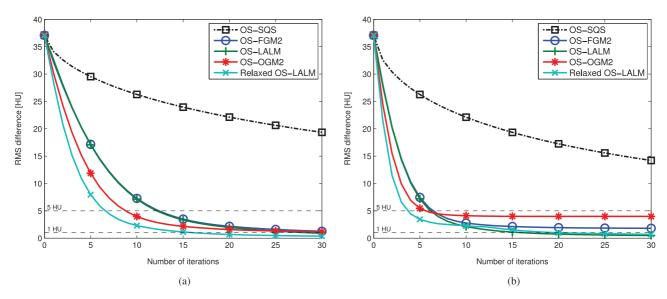
Fig. 5. Chest: Convergence rate curves of different OS algorithms with (a) 10 subsets and (b) 20 subsets. The proposed relaxed OS-LALM with 10 subsets exhibits similar convergence rate as the unrelaxed OS-LALM with 20 subsets. (a) 10 subsets, (b) 20 subsets.
