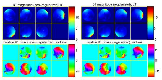
Fig. 3. Estimated  $B_1$  magnitude (top) and phase (bottom) maps by the nonregularized method (left) and the regularized method (right), in phantom study.
