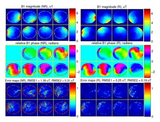
Fig. 2. Estimated  $B_1$  magnitude (top row), phase (middle row) maps, and the error (bottom row) maps by the nonregularized (NR) method (left) and the regularized (R) method (right) using conventional all-but-one coil combination scans, in simulation study.
