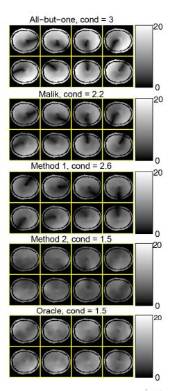
Fig. 6. Magnitude of the composite  $B_1$  maps (masked),  $\bar{B}_n(r)$ , by different methods, in  $\mu$ T. Condition numbers (cond) of the coil combination matrices are shown on the titles.
