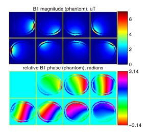
Fig. 4.  $B_1$  maps of the phantom (masked by the brain shape), used for optimizing the coil combinations.
