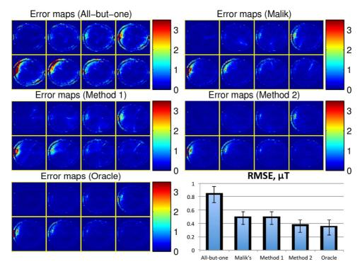
Fig. 8. Error maps of the estimated complex  $B_1$  maps (in  $\mu$ T) of all the methods and the corresponding RMSEs.
