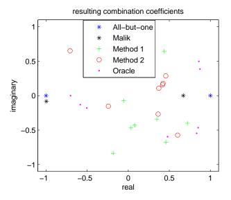
Fig. 5. The first row of the coil combination matrices designed by different methods, where the magnitude is normalized to the peak nominal power of the system.
