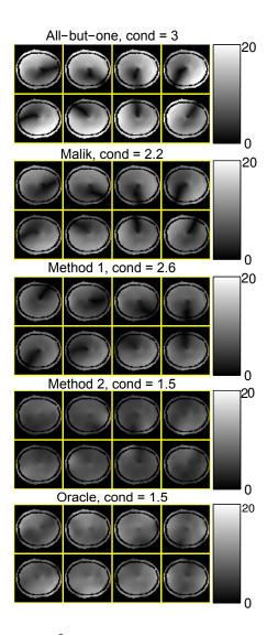
Fig. 6. Magnitude of the composite  $B_1$  maps (masked),  $\tilde{B}_n(r)$ , by different methods, in  $\mu T$ . The condition numbers (cond) of the coil combination matrices are shown on the titles.
