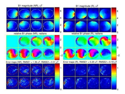
Fig. 2. The estimated  $B_1$  magnitude (top row), phase (middle row) maps and the error (bottom row) maps by the non-regularized (NR) method (left) and the regularized (R) method (right) using conventional all-but-one coil combination scans, in simulation study.
