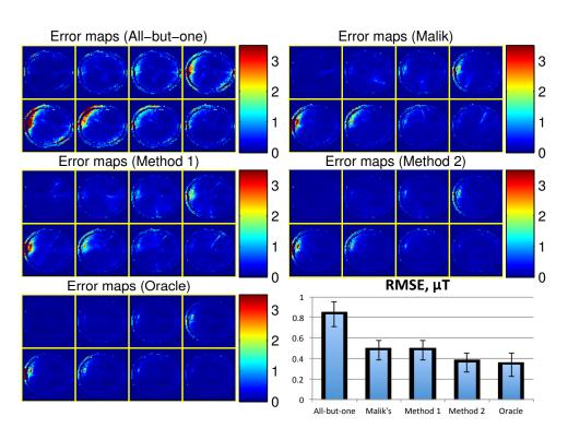
Fig. 8. The error maps of the estimated complex  $B_1$  maps (in  $\mu$ T) of all the methods and the corresponding RMSEs.
