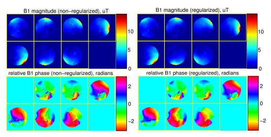
Fig. 3. The estimated  $B_1$  magnitude (top) and phase (bottom) maps by the non-regularized method (left) and the regularized method (right), in phantom study.
