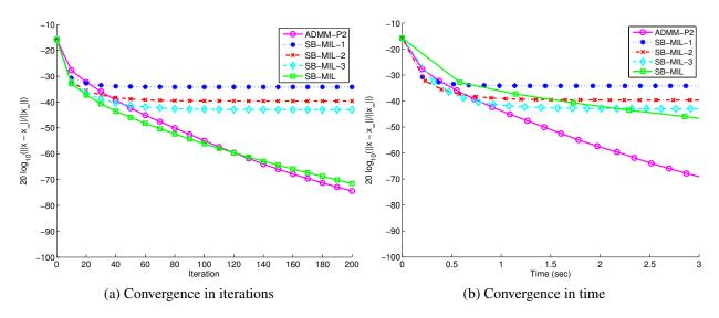
Figure 6: Experiment 1: BSNR = 40dB, Uniform  $9 \times 9$  blur. Convergence speed of ADMM-P2 and variations of SB-MIL with 4 inner CG iterations compared to the solution of P1  $\mathbf{x}^{(\infty)}$  (eq (11) in manuscript). The number in SB-MIL-X denotes the number of outer iterations that CG is applied. SB-MIL denotes the version of the algorithm where CG is applied in all outer iterations. The previous convention is followed in all subsequent figures.
