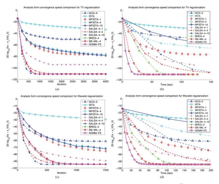
Fig. 4. Experiment 3: algorithm convergence speed results with convergence measured in terms of drop in NRMSE in dB,  $\xi^{(k)}$ , between the estimated image  $\hat{\mathbf{x}}$  and the converged image  $\mathbf{x}^{(\infty)}$ . Left column (a,c) is convergence per iteration and right column (b,d) is convergence in run-time. First row (a,b) is from TV regularizer and second row (c,d) is from wavelet  $l_1$ -norm regularizer.
