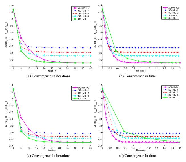
Figure 11: Experiment 3: BSNR = 50dB, 15 pixel motion blur. Convergence speed of ADMM-P2 and variations of SB-MIL with 4 (a, b) and 10 (c, d) inner CG iterations compared to the true image  $x_{true}$ .
