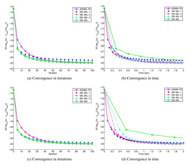
Figure 9: Experiment 2: BSNR = 50dB, Uniform  $15 \times 15$  blur. Convergence speed of ADMM-P2 and variations of SB-MIL with 4 (a, b) and 10 (c, d) inner CG iterations compared to the true image  $x_{true}$ .
