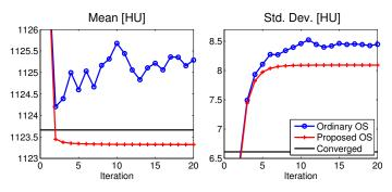
Fig. 4. GE performance phantom: mean and standard deviation within a uniform region in the first slice of the ROI (see Fig. 3) vs. iteration, showing the instability of ordinary OS approach with 328 subsets, compared with the proposed OS approach. Also shown is the result from a converged image  $x^{(\infty)}$  generated from several iterations of a convergent algorithm.
