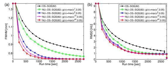
Fig. 5. GE performance phantom: plots of (a) FWHM and (b) RMSD as a function of run time for different choice of DRA parameters t for  $\epsilon = 0.05$ . The plot markers show each iteration. There are no changes during first iterations, since we consider precomputing the denominator using one forward and back projections as one iteration.
