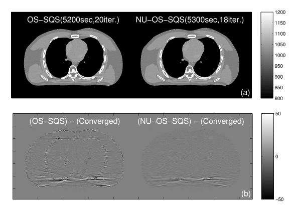
Fig. 4. A simulated XCAT phantom: (a) A center slice of reconstructed image by OS-SQS(82) and NU-OS-SQS(82)- $g(v) = \max\{v^{10}, 0.05\}$  after about 88 min. (b) Difference between the reconstructed and converged images are additionally shown to illustrate the acceleration of NU approach. (Images are cropped for better visualization.)
