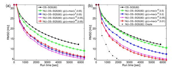
Fig. 6. A shoulder region scan: plot of RMSD versus run time for different choice of parameters (a) t and (b)  $\epsilon$  in  $g(v) = \max\{v^t, \epsilon\}$ .
