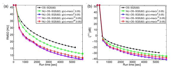
Fig. 3. A simulated XCAT phantom: plots of (a) RMSD and (b)  $\xi^{(n)}$  versus run time for different choice of parameters t for  $\epsilon = 0.05$  in  $g(v) = \max\{v^t, \epsilon\}$ .
