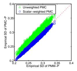
Fig. 5. If the spatial resolutions are matched, the SD of PMC is higher than or comparable to the SD of PMM, depending on the choice of weights  $\alpha_m$ .
