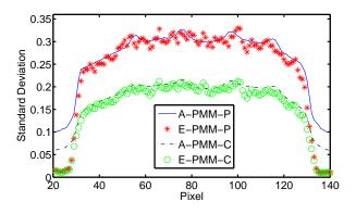
Fig. 4. Analytical SD of PMM (A-PMM-P, A-PMM-C) matches well with empirical SD of PMM (E-PMM-P, E-PMM-C), respectively.
