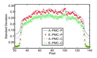
Fig. 3. Analytical SD of PMC (A-PMC-P, A-PMC-C) matches well with empirical SD of PMC (E-PMC-P, E-PMC-C), respectively.
