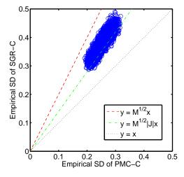
Fig. 6. Empirical SD of SGR vs. empirical SD of PMC (MCIR) with 4 frames (M = 4). The SD of PMC will be affected by *both* the number of frames and the motion (Jacobian determinant of transformation |J|).
