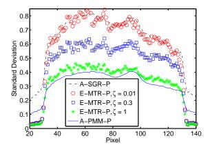
Fig. 11. Empirical SD of MTR with different  $\zeta$ . As  $\zeta \to 0$ , the SD of MTR approaches to the analytical SD of SGR. As  $\zeta \to \infty$ , the SD of MTR approaches to the analytical SD of PMM.
