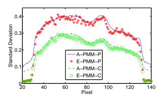
Fig. 10. Analytical SD of PMM (A-PMM-P, A-PMM-C) matches well with empirical SD of PMM (E-PMM-P, E-PMM-C), respectively.
