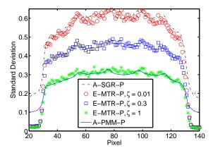
Fig. 7. Empirical SD of MTR with different  $\zeta$ . As  $\zeta \to 0$ , the SD of MTR approaches the analytical SD of SGR. As  $\zeta \to \infty$ , the SD of MTR approaches the analytical SD of PMM.
