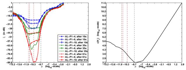
Fig. 4. Experiment with Slice 38 of *in-vivo* human brain data-set (corresponding to Section V-C): Plots of  $\xi$  for various run-times of AL-P1 and condition number  $\kappa(\mathbf{G}_{\mu})$  as functions of  $\mu$ . It is seen that AL-P1 using  $\mu_{\min}$  (indicated by a black-dashed line) converges relatively slowly compared to using  $\mu_{\text{opt}}$ .
