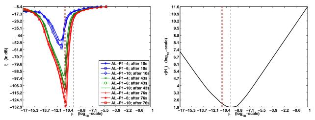
Fig. 7. Experiment with modified synthetic data-set: Plots of  $\xi$  for various run-times of AL-P1 and condition number  $\kappa(\mathbf{G}_{\mu})$  as functions of  $\mu$ . The  $\mu$  that minimizes  $\kappa(\mathbf{G}_{\mu})$  does not yield the best convergence speed for AL-P1.
