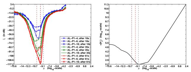
Fig. 5. Experiment with Slice 90 of *in-vivo* human brain data-set (corresponding to Section V-C): Plots of  $\xi$  for various run-times of AL-P1 and condition number  $\kappa(\mathbf{G}_{\mu})$  as functions of  $\mu$ . It is seen that AL-P1 using  $\mu_{\min}$  (indicated by a black-dashed line) converges relatively slowly compared to using  $\mu_{\text{opt}}$ .
