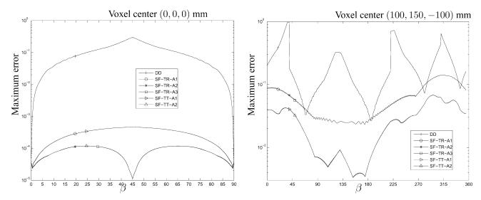
Fig. 3. Maximum error comparison between the forward DD, SF-TR, and SF-TT projector for a voxel centered at the origin (left) and a voxel centered at (100, 150, -100) mm (right).
