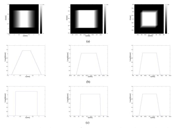
Fig. 2. Exact footprint functions  $q(s, t; \beta; \vec{n})$  and their profiles for 1 mm<sup>3</sup> voxels centered at the origin (left), (100, 150, 15) mm (center), and (93, 93, 93) mm (right). (a) True footprint. (b) Profile in s. (c) Profile in t.
