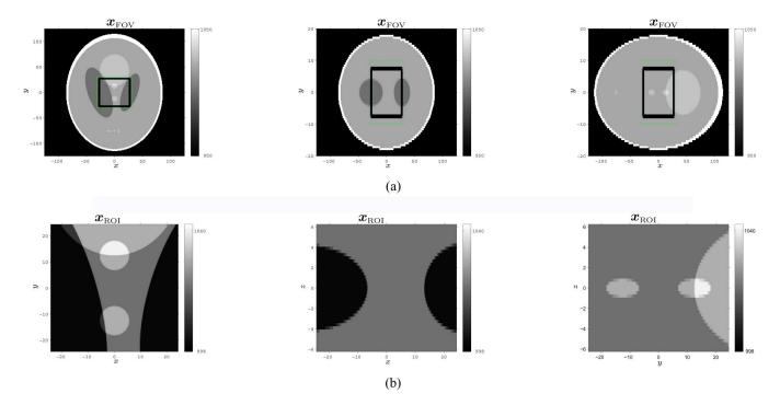
Fig. 4. Shepp-Logan digital phantoms in Hounsfield units. The first, second, and third columns show axial, coronal, and sagittal views, respectively. (a) FOV images. (b) ROI images. The black rectangular box shows the transition zone. The green lines show the region of ROI reconstruction.
