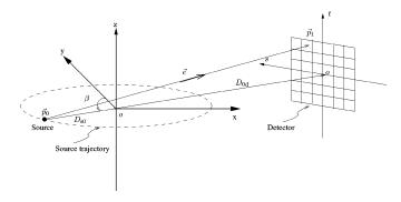
Fig. 1. Axial cone-beam flat-detector geometry.
