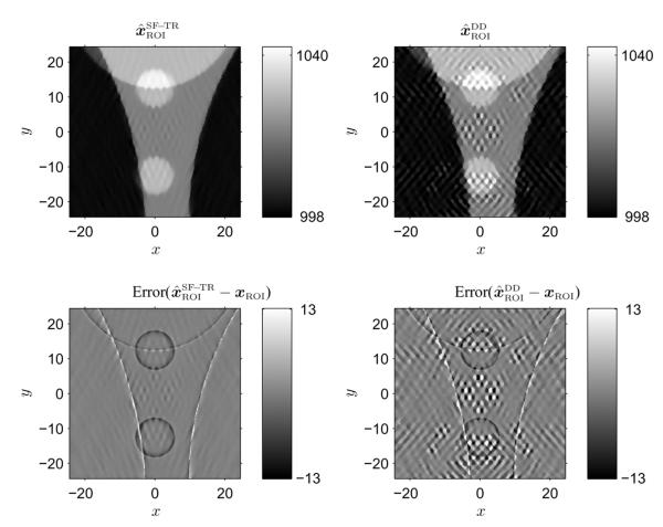
Fig. 6. Axial views of ROI images  $\hat{x}_{ROI}^{SF-TR}$  and  $\hat{x}_{ROI}^{DD}$  reconstructed by the iterative method (PWLS-CG) using the SF-TR and DD method, respectively. Left: SF-TR projector. Right: DD projector.
