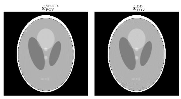
Fig. 5. Axial views of FOV images  $\hat{x}_{FOV}^{SF-TR}$  and  $\hat{x}_{FOV}^{DD}$  reconstructed by the iterative method (PWLS-CG) using the SF and DD method, respectively. Left: SF-TR projector. Right: DD projector.
