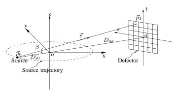
Fig. 1. Axial cone-beam flat-detector geometry.
