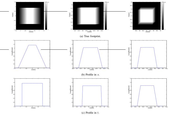
Fig. 2. Exact footprint functions  $q(s, t; \beta; \vec{n})$  and their profiles for 1mm<sup>3</sup> voxels centered at the origin (left), (100, 150, 15) mm (center) and (93, 93, 93) mm (right).
