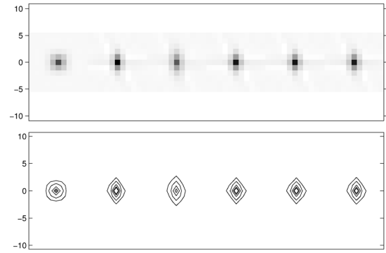
Fig. 10. Impulse Responses at (-100, -100) . From left to right, target, conventional regularization, certainty based regularization, AIMA regularization with \alpha = 0.1 , AIMA regularization with \alpha = 0 , FIIN regularization with \alpha = 0 .
