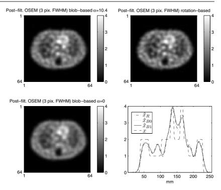
**Figure 5.** A slice and profiles through over-iterated and post-smoothed OSEM-reconstructed images of a single realization of the noisy data. Superimposed on the profile of the true high-resolution phantom (x) are those of the images reconstructed with the rotation-based model  $(\hat{x}_R, \text{NMSE} = 4.12\%)$ , the blob-based model with  $\alpha = 0$   $(\hat{x}_{B0}, \text{NMSE} = 2.99\%)$  and the blob-based model with  $\alpha = 10.4$   $(\hat{x}_{B1}, \text{NMSE} = 3.60\%)$ .
