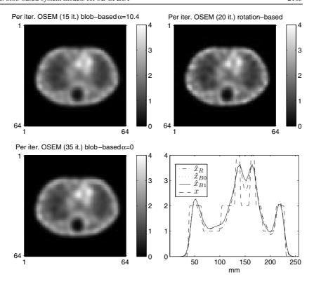
**Figure 4.** A slice and profiles through OSEM-reconstructed images of a single realization of the noisy data. Superimposed on the profile of the true high-resolution phantom (x) are those of the images reconstructed with the rotation-based model  $(\hat{x}_R, \text{NMSE} = 3.26\%)$ , the blob-based model with  $\alpha = 0$  ( $\hat{x}_{B0}$ , NMSE = 2.76%) and the blob-based model with  $\alpha = 10.4$  ( $\hat{x}_{B1}$ , NMSE = 2.87%).
