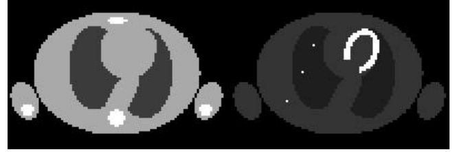
Fig. 3. Attenuation map (left) and activity distribution (right) for the simulated thorax phantom. The points are numbered from bottom to top, the first point (in tissue) is used to determine the local impulse response.
