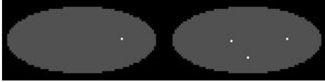
Fig. 2. Simulation objects to compare uniform resolution penalized-likelihood reconstruction to post-smoothed MLEM. Left: the object used to determine the local impulse response. Right: two more points were added for the signal-to-noise ratio measurement.
