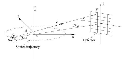
Figure 2.2: Axial cone-beam flat-detector geometry.
