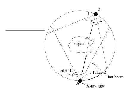
Figure 4.1: Schematic diagram of a fan-beam CT scanner with two positions of X-ray source and split-filter assembly.
