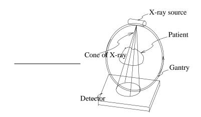
Figure 2.1: Schematic diagram of a X-ray scanner.
