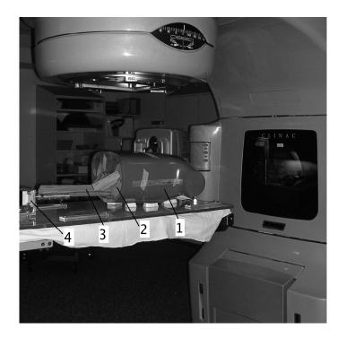
Figure 3.18: A picture of the movable phantom: 1. the phantom; 2. the diaphragm; 3. the wood connector; 4. the actuator.
