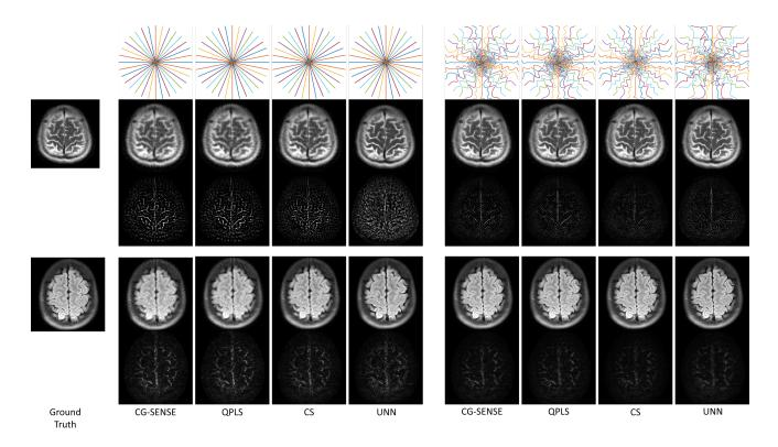
Fig. 4. Examples of the reconstructed images with unoptimized (left) and optimized trajectories (right). The third row shows corresponding error maps.
