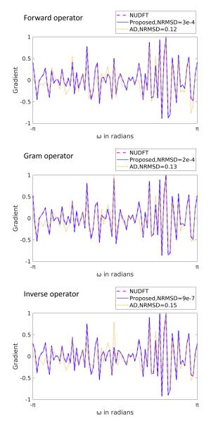
Fig. 2. Examples of gradients w.r.t.  $\omega$ . Plots show one spoke of 80 points (rescaled to [-1,1]). The rows are the forward, Gram, and 'inverse of PSD' operator cases. The proposed approximation better matches the gradient of the NUDFT. The bottom left corner of each plot shows the normalized root-mean-square difference (NRMSD) compared with the NUDFT calculation.
