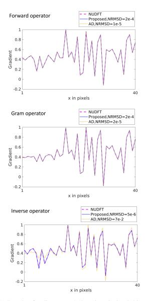
Fig. 1. Examples of gradients w.r.t.  $\boldsymbol{x}^*$  (the real part is plotted). Plots show one representative row of a 40 × 40 matrix (rescaled to [-1,1]). The rows are the forward, Gram, and 'inverse of PSD' operator cases. Three calculation methods (in three columns) achieve very similar results. The horizontal axis is the pixel index. The bottom left corner of each plot shows the normalized root-mean-square difference (NRMSD) compared with the reference NUDFT calculation.
