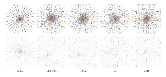
Fig. 3. Optimized sampling trajectories for several iterative reconstruction methods. The left column shows the uniform radial initialization. The second row shows the  $8 \times$  zoomed-in central k-space.
