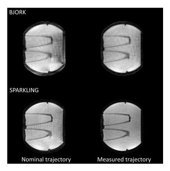
Fig. S1. CS-based reconstruction of a water phantom. The left column is the reconstruction with the nominal trajectory, and right is with the measured trajectory. Reconstruction with the mapped trajectory introduces fewer artifacts.
