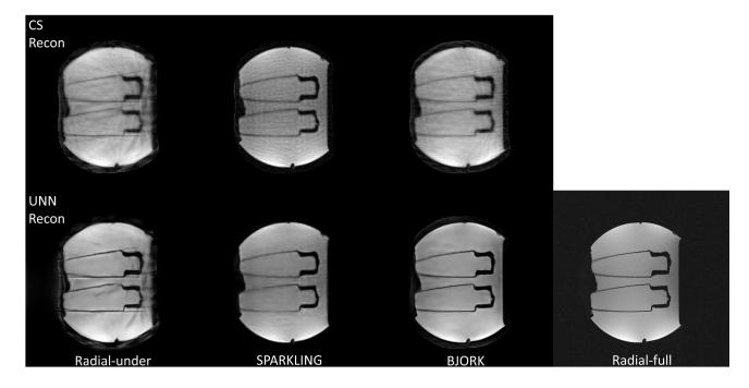
Fig. 6. Representative results of the phantom experiment using CS-based and UNN-based reconstruction algorithms. The sequences involved were radial-like GRE (detailed in Table I). The readout length was 2.56 ms, and we used 16/320 spokes for undersampled (Radial-Under, SPARKLING, BJORK) trajectories and the fully-sampled radial trajectory.
