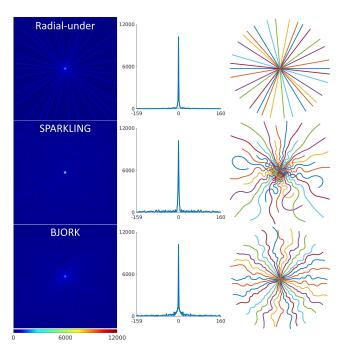
Fig. 2. PSFs of different sampling patterns. The plots show the magnitude of the row across the zero point.
