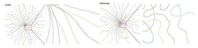
Fig. S2. The measurement of the influence of the eddy currents on readout waveform. The solid line is the nominal trajectory, and the dotted line is the measurement.
