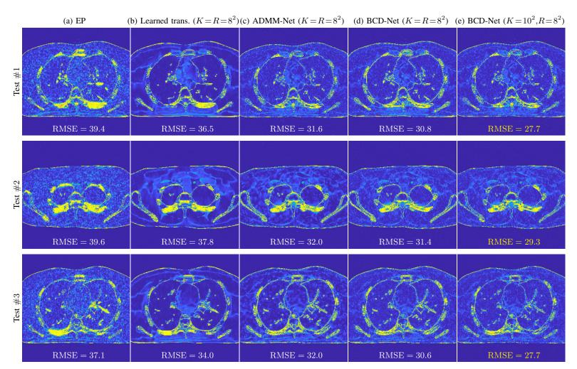
Fig. S.3. Error images of three reconstructed XCAT phantom images with different MBIR methods (images are magnified to better show differences; display window is [0, 100] HU; and RMSE values are in HU).
