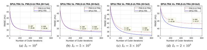
Fig. 3: RMSE comparison of SPULTRA and PWLS-ULTRA. The cursors indicate the RMSEs (Y) at specific number of outer iterations (X).
