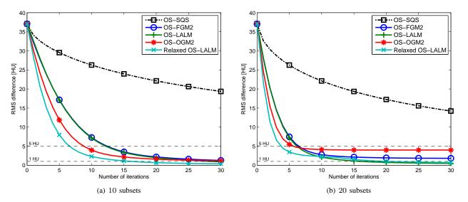
Fig. 5: Chest: Convergence rate curves of different OS algorithms with (a) 10 subsets and (b) 20 subsets. The proposed relaxed OS-LALM with 10 subsets exhibits similar convergence rate as the unrelaxed OS-LALM with 20 subsets.
