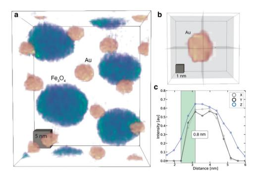
Fig. 2. Measuring 1nm Resolution for Au-Fe<sub>3</sub>O<sub>4</sub> Nanoparticles. **a**, Fused EELS tomograms of Au-Fe<sub>3</sub>O<sub>4</sub> nanoparticles. **b,c**, Line scan profiles of a 2.5 nm Au nanoparticle gives a resolution of 0.8, 0.8 and 1.2 nm along the x, y, and z directions.
