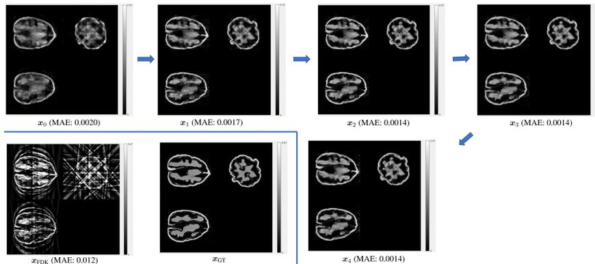
Figure 2: Center-slices along  $x$ - $y$ ,  $y$ - $z$ , and  $x$ - $z$  directions from the reconstruction of a test walnut across various stages ( $x_1 - x_4$ ) using the proposed method. The ground truth using a full set of views ( $x_{GT}$ ) and FDK reconstruction using only 8 views ( $x_{FDK}$ ) have been shown in the bottom left. The initialization for our method has been depicted on top left ( $x_0$ ). Mean absolute errors (MAE) are shown, wherever applicable.
