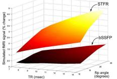
Figure 3: Monte Carlo Bloch simulation results: Percent functional signal change for STFR and bSSFP as a function of TR (7-14 ms) and flip angle (12-24° – the bSSFP flip angle is twice the value indicated). STFR fMRI is predicted to produce 3-5 fold signal increase relative to passband bSSFP.
