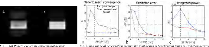
*Fig.* 2: (a) Pattern excited by conventional design; (b) pattern excited by joint design, which effectively adjusts phase encoding (Fig. 1) to reduce aliasing.
