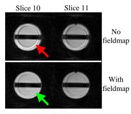
Figure 1: 2 slices of a resolution phantom collected using the 3D FSE. Top two images have no field map in the reconstruction and the bottom 2 include field map.
