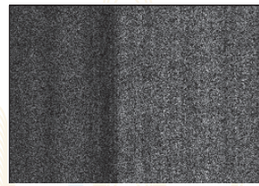
Synthetic aperture radar image that is defocused due to phase errors.
