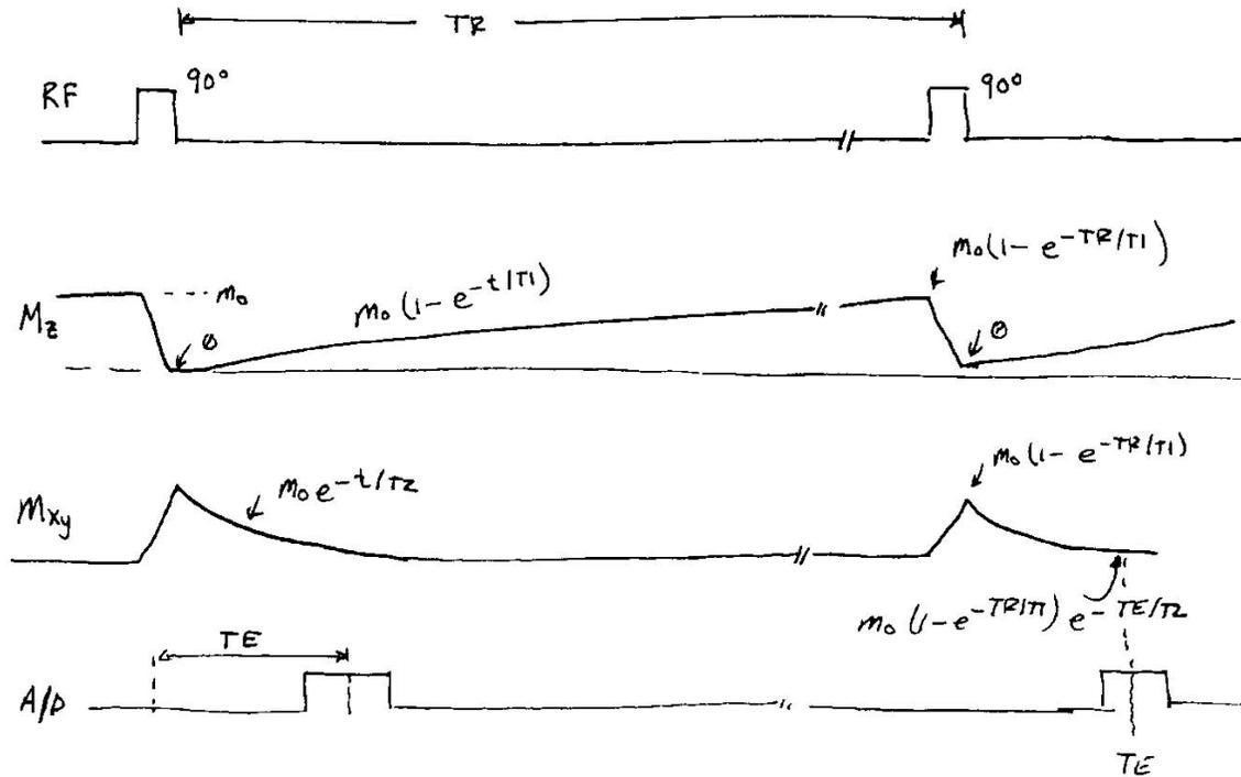
**Steady State Magnetization for  $\alpha$  pulses**
