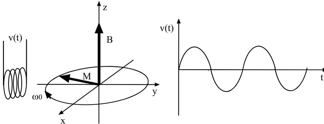
If we place a small loop of wire near this precessing magnetization, we will induce a voltage in the coil,  $v(t)$ , at frequency,  $\omega_0 = \gamma B_0$ .
