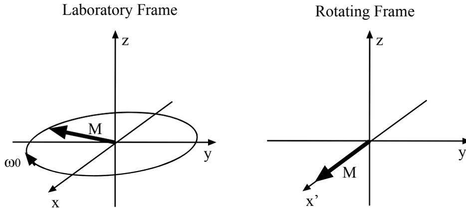
Conceptually, we can think of this as being similar to riding on a carousel. If we are on the carousel, other objects on the carousel appear stationary, but to someone on the ground, the objects are spinning by at  $\omega_{\text{carousel}} = \omega_0$ .
