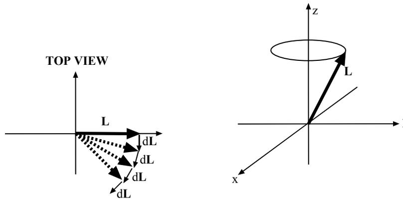
These relationship works out so that the top precesses around the gravitational field. It can be shown that the precession frequency is:
