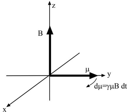
Given that the circumference of the circle here is  $2\pi\mu$ , the time for one cycle of precession is  $2\pi\mu/\gamma\mu B$ , and the frequency of precession is thus,  $f = \gamma B/2\pi$  or  $\omega = \gamma B$ . The latter is the most important relationship in NMR and MRI. It is known as the Larmor relationship:
