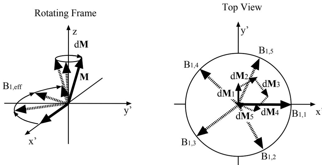
Under this condition, the  $\mathbf{M}$  vector never gets far from the z-axis because the  $\mathbf{B}_1$  vector moves to a position that causes the change in  $\mathbf{M}$  (e.g.  $d\mathbf{M}$ ) to move back towards the z-axis.
