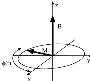
The direction that the  $\mathbf{M}$  points (the phase of  $\mathbf{M}$ ) is given by the time integral of the frequency function:
