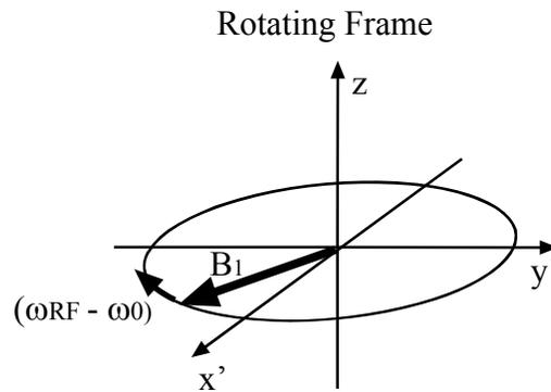
In this case, as  $\mathbf{M}$  gets tipped away from the z-axis  $\mathbf{B}_1$  has moved relative the  $\mathbf{M}$  and the axis of rotation has now changed.
