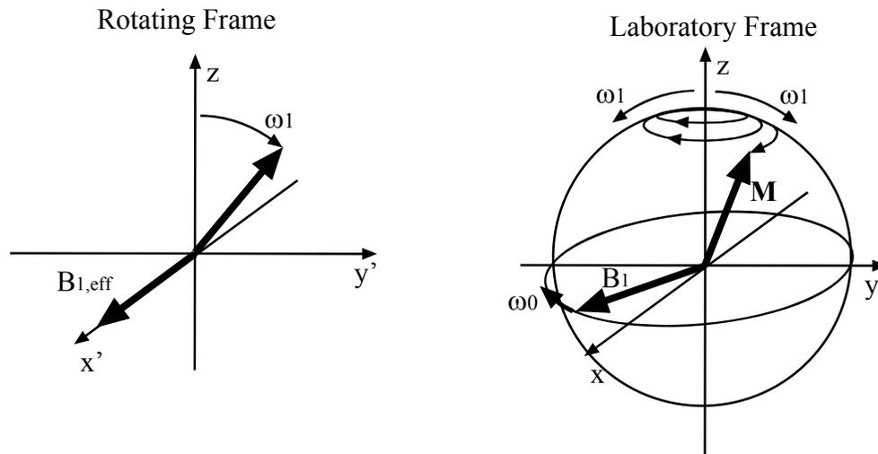
If we go back to the lab frame, then motion of  $\mathbf{M}$  is rather complex – simultaneously precessing about  $\mathbf{B}_1$  at  $\omega_1$  and about  $B_0 \mathbf{k}$  at  $\omega_0$ . Using the relationships that related rotating frame to lab frame we get:
