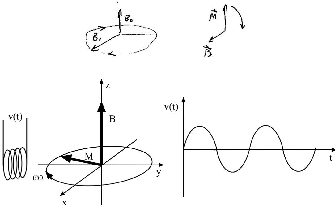
3. Gradient magnetic fields are applied to set-up a one-to-one correspondence between spatial position and frequency. For example, if we apply an  $x$  gradient,  $G_x$ , the magnetic field distribution is:  $B(x) = B_0 + G_x \cdot x$ , and thus:
