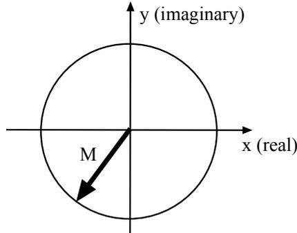
Now, let's consider a non-constant  $\mathbf{B}$ :  $\mathbf{B}(t) = [B_0 + \Delta B(t)]\mathbf{k}$  (the  $\mathbf{B}$  field is still applied along the z-axis). As before,  $\mathbf{M}$  will still precess around  $\mathbf{B}$ , but now the frequency of precession will vary with time:
