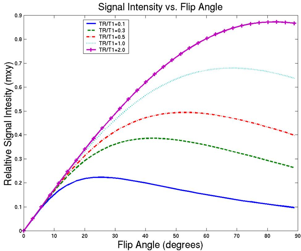
The above relationship can be differentiated to yield the optimal  $\alpha$  (in terms of maximal signal):
