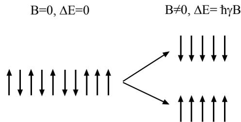
The energy difference between these states is determined by the strength of the applied magnetic field, which we will call  $B_0$ , in the following relationship:
