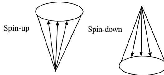
The spin and magnetic moment exist in all directions simultaneously, but average behavior is non-zero in only one of the directions:
