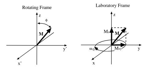
2. 180 degree or π pulses. Here the RF pulses is applied for a duration and amplitude that leads to a precession angle, f, of 180 degrees. There are two variants of 180 degree pulses: inversion and spin-echo pulses. In an inversion pulse, M starts aligned to the z axis and is inverted to the -z axis. In an spin-echo pulse, M starts in the x'-y' plane and is flipped (around the axis of B<sub>1</sub>) to a new position in the x'-y' plane. We'll talk more about both of
