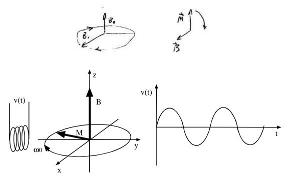
3. Gradient magnetic fields are applied to set-up a one-to-one correspondence between spatial position and frequency. For example, if we apply an *x* gradient,  $G_x$ , the magnetic field distribution is:  $B(x) = B_0 + G_x x$ , and thus:
