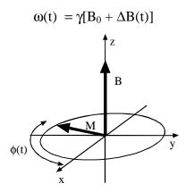
The direction that the M points (the phase of M) is given by the time integral of the frequency function:
