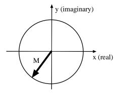
Now, let's consider a non-constant **B**:  $\mathbf{B}(t) = [\mathbf{B}_0 + \Delta \mathbf{B}(t)]\mathbf{k}$  (the **B** field is still applied along the z-axis). As before, **M** will still precess around B, but now the frequency of precession will vary with time:
