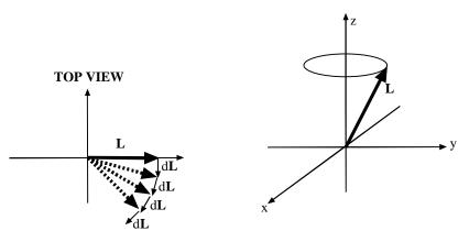
These relationship works out so that the top precesses around the gravitational field. It can be shown that the precession frequency is:
