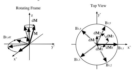
Under this condition, the **M** vector never gets far from the z-axis because the  $B_1$  vector moves to a position that causes the change in **M** (e.g. d**M**) to move back towards the z-axis.
