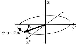
In this case, as M gets tipped away from the z-axis  $B_1$  has moved relative the M and the axis of rotation has now changed.
