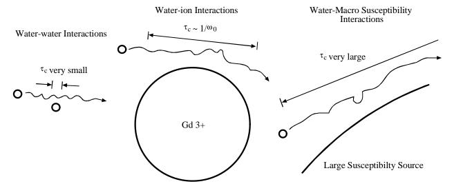
In general, T1 properties result from a complex interaction of different mechanisms with different kinds of spin motion. Here are some factors that influence T1:
