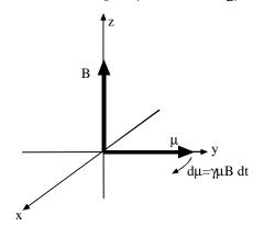
Given that the circumference of the circle here is  $2\pi\mu$ , the time for one cycle of precession is  $2\pi\mu/g\mu B$ , and the frequency of precession is thus,  $f = gB/2\pi$  or  $\omega = gB$ . The latter is the most important relationship in NMR and MRI. It is known as the Lamor relationship:
