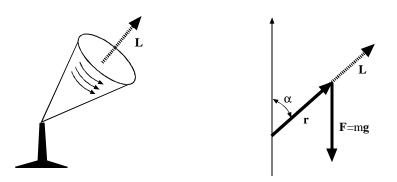
In this drawing, the force generated by the mass of the top and the gravitational field ( $\mathbf{F} = m\mathbf{g}$ ) appears to be acting at the center of mass of the top, which is located at position  $\mathbf{r}$ , a distance r from the tip of the top. The angular momentum of the top is  $\mathbf{L}$  ( $\mathbf{F}$ ,  $\mathbf{L}$ ,  $\mathbf{g}$ , and  $\mathbf{r}$  are all vector quantities). The simplified equation of motion for this top, describes the torque on the angular momentum:
