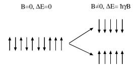
The energy difference between these states is determined by the strength of the applied magnetic field, which will we will call  $B_0$ , in the following relationship:
