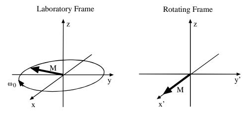
Conceptually, we can think of this as being similar to riding on a carousel. If we are on the carousel, other objects on the carousel appear stationary, but to someone on the ground, the objects are spinning by at  $w_{\text{carousel}} = w_0$ .
