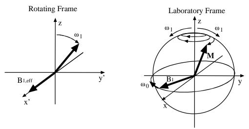
If we go back to the lab frame, then motion of M is rather complex – simultaneously precessing about **B**<sub>1</sub> at  $\omega_1$  and about B<sub>0</sub>**k** at  $\omega_0$ . Using the relationships that related rotating frame to lab frame we get:
