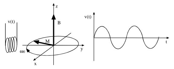
If we place a small loop of wire near this precessing magnetization, we will induce a voltage in the coil, v(t), at frequency,  $\omega_0 = \gamma B_0$ .
