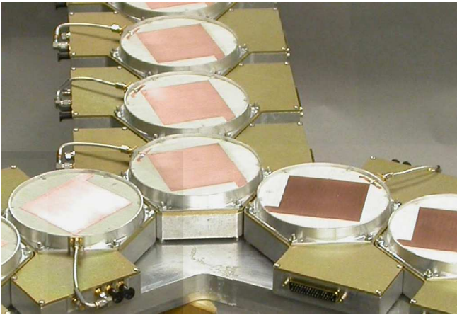
Figure 6. A close-up of the previous Figure, showing the three orientations of the receivers, with one orientation per leg. Each antenna has a fixed orientation with respect to its receiver. Since each antenna is left circularly polarized, rather than linearly polarized, the polarization states remain aligned regardless of antenna orientation.
