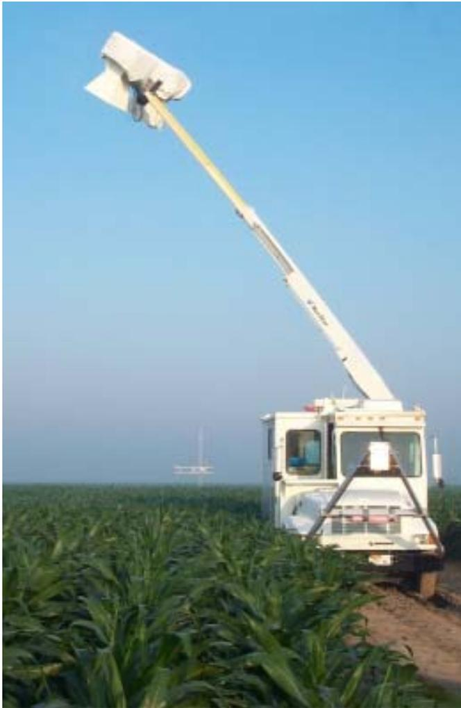
Fig. 1. Truck-mounted radiometers on day of year 178. Antennae oriented at  $\theta = 35^\circ, \phi = 60^\circ$ . Micro-meteorological station tower can be seen in the background.
