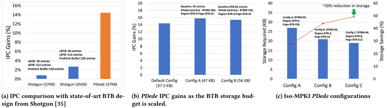
Figure 12: PDede IPC sensitivity at larger sizes, in future cores and storage savings possible at Iso-MPKI
