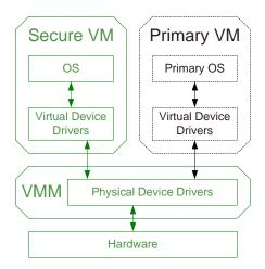
**Figure 1.** In the Storage Capsule architecture, the user's primary operating system runs in a virtual machine. The secure VM handles encryption and declassification. The dotted black line surrounding the primary VM indicates that it is *not* trusted. The other system components are trusted.
