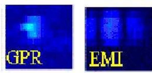
Figure 4.3: Signatures from a mid-depth, metal cased landmine.
