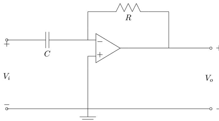
Figure 3.2.2: Differential Controller
