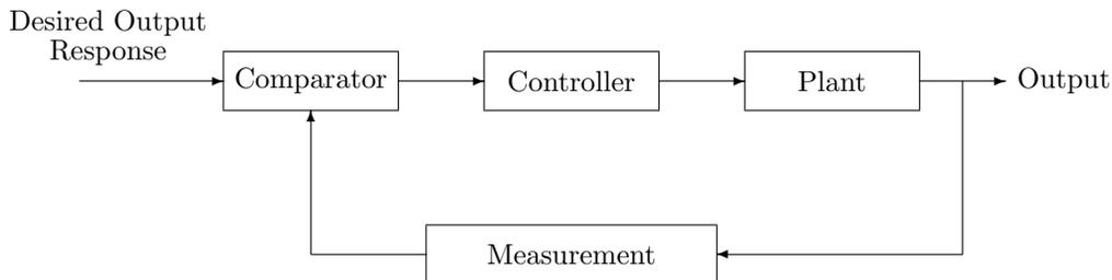
Figure 1.0.1: Closed-Loop Control System. The plant is the generic term for the system to be controlled.
