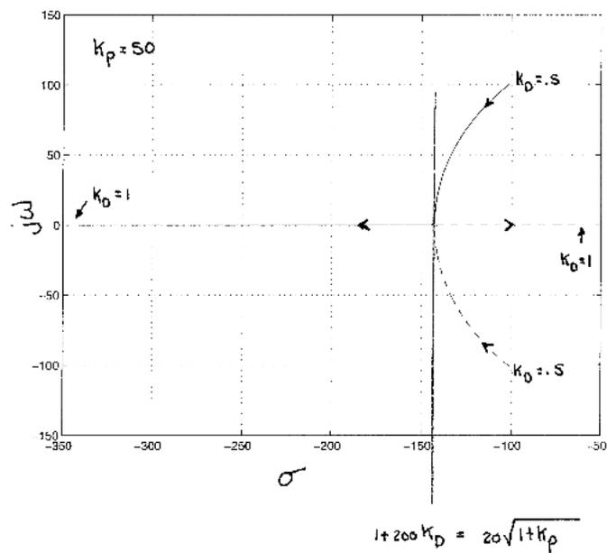
Figure 3.4.1: Root-locus plot of PD controller with 2 degrees of freedom
