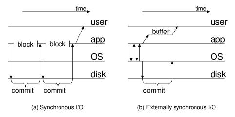
This figure shows the behavior of a sample application that makes two file system modifications, then displays output to an external device. The diagram on the left shows how the application executes when its file I/O is synchronous; the diagram on the right shows how it executes when its file I/O is externally synchronous.
