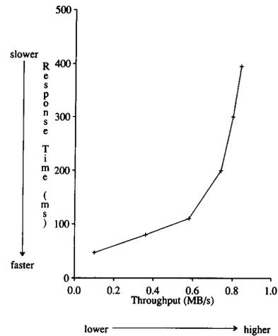
Fig. 2. Example response time versus throughput graph. Increasing the utilization of a system usually leads to higher throughput but slower response time. This figure was adapted from [6].
