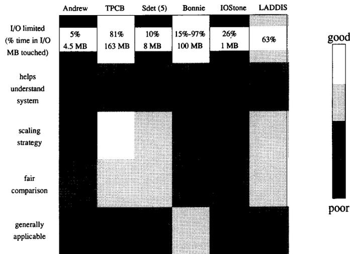
Fig. 15. Current state of I/O benchmarks. In this figure, we show a qualitative evaluation of benchmarks used today to evaluate I/O systems. We see that several are not I/O-bound and that most do not provide understanding of the system, lack a well-defined scaling strategy, and are not generally applicable. The percent time spent in I/O was measured on the DECstation 5000/200 of Fig. 7.
