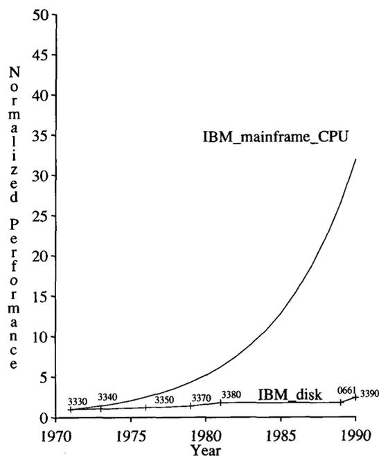
**Fig. 1.** Contrasting trends of CPU and disk performance improvements. Over the past two decades, CPU performance improvements have far outstripped disk performance improvements. In this graph, CPU performance refers to IBM mainframe performance; disk performance refers to IBM disk (33×0 series) throughput on a random 8-kb access. Both are normalized to their 1971 level. The IBM mainframe performance comes from [18, p. 4, fig.1.1].
