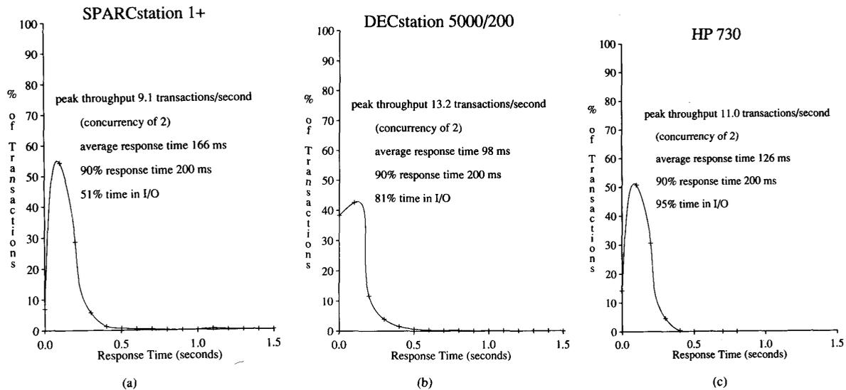
Fig. 9. TPC-B Results. These figures show TPC-B results for our three experimental systems. As a database program, we used Seltzer's simple transaction processing library LIBTP [57]. Due to software limitations, we were unable to run at concurrencies higher than 2, reflected by response times much faster than those required by TPC-B.
