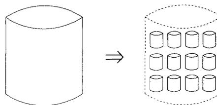
Fig. 5. Combining multiple smaller disks to improve performance. Performance of single disks is not improving rapidly (Fig. 4); however, disks are rapidly becoming physically smaller and cheaper. Disk arrays take advantage of this downsizing to provide higher aggregate throughput by simultaneously operating many small disks.
