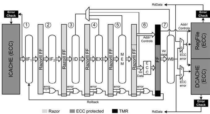
Figure 22.1.3: Razor II enabled 64-bit Alpha processor architecture.
