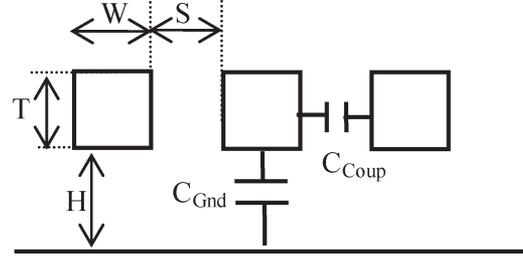
Fig. 2. Cross section of a generic interconnect structure.
