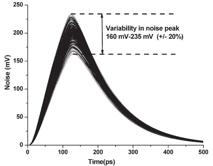
Fig. 9. Crosstalk-noise waveforms as obtained by Monte Carlo simulations. Nominal values (three-sigma tolerances) for metal width, thickness, and ILD height were  $0.4 \mu\text{m}$  (25%),  $0.75 \mu\text{m}$  (21%), and  $0.3 \mu\text{m}$  (17%), respectively. Nominal interwire spacing was  $0.45 \mu\text{m}$  and it was inversely correlated with width.
