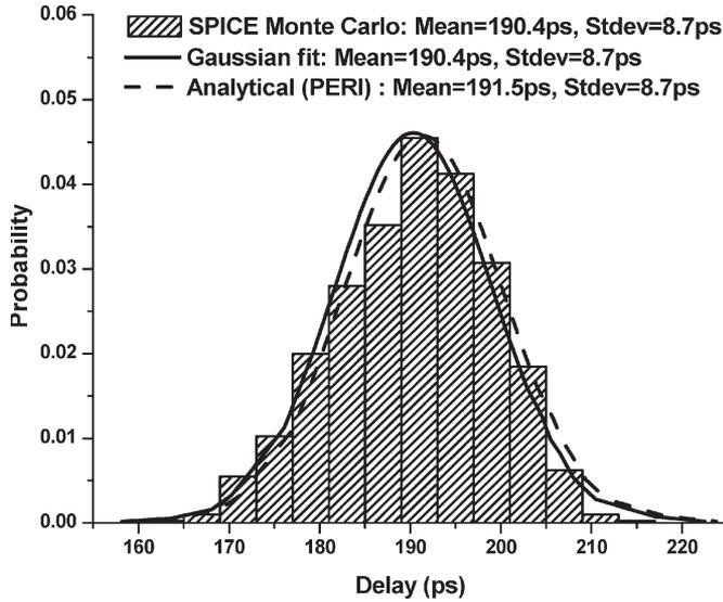
Fig. 8. Analytical delay distribution for saturated ramp input obtained using the statistical PERI method compared to Monte Carlo simulations. The Gaussian-fit curve shows Gaussian fitting to the HSPICE mean and standard deviation. Nominal values (three-sigma tolerances) for metal width, thickness, and ILD height were  $0.5 \mu\text{m}$  (13%),  $0.4 \mu\text{m}$  (16%), and  $0.3 \mu\text{m}$  (19%), respectively.
