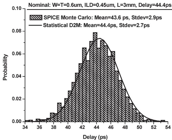
Fig. 18. Analytical delay distribution obtained using statistical D2M metric compared to Monte Carlo simulations. Nominal values (three-sigma tolerances) for metal width, thickness, and ILD height were 0.6 μm (30%), 0.6 μm (30%), and 0.45 μm (30%), respectively.
