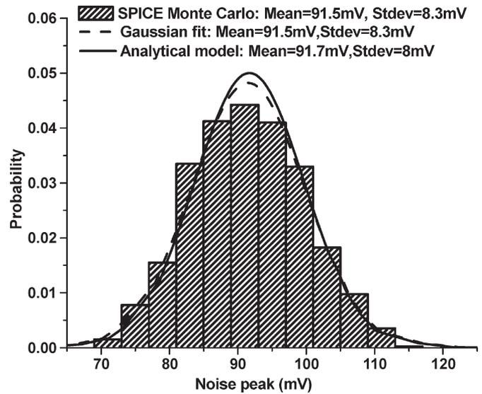
Fig. 12. Analytical noise-peak distribution compared to Monte Carlo simulations. The Gaussian-fit curve shows Gaussian fitting to the HSPICE mean and standard deviation. Nominal values (three-sigma tolerances) for metal width, thickness, and ILD height were 0.55 μm (14%), 0.44 μm (30%), and 0.3 μm (15%), respectively. Nominal interwire spacing was 0.4 μm and it was inversely correlated with width.
