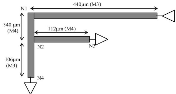
Fig. 20. Topology of a physical net taken from an industrial design.
