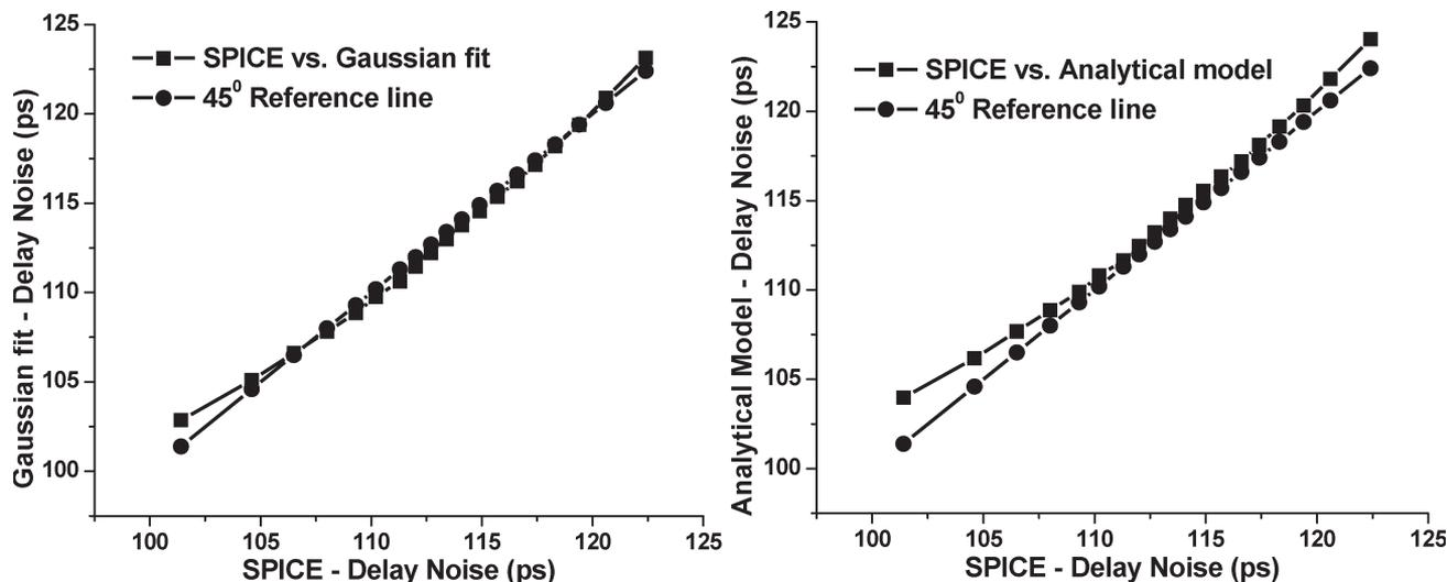
Fig. 17. q-q plots for dynamic delay: (Left) HSPICE results versus Gaussian distribution (with same mean and standard deviation as obtained from SPICE simulations) with 45° reference line. (Right) SPICE result versus analytical model with 45° reference line. Nominal values (three-sigma tolerances) for metal width, thickness, and ILD height were 0.65 μm (23%), 0.5 μm (11%), and 0.26 μm (11%), respectively. Nominal interwire spacing was 0.4 μm and it was inversely correlated with width.
