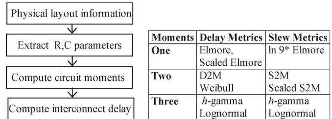
Fig. 1. Moment-based-delay-modeling flow and some existing nominal delay and slew metrics as available in literature.
