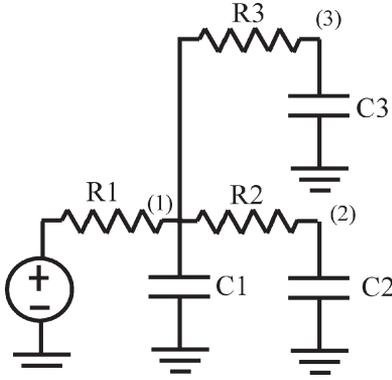
Fig. 3. Simple RC tree.
