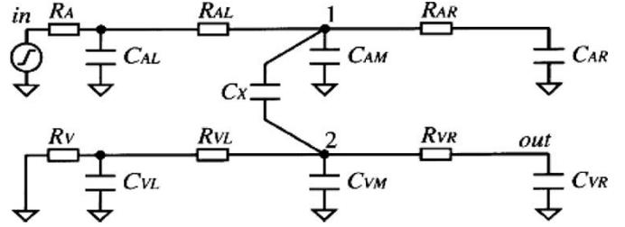
Fig. 10. Six-node circuit template for coupling noise estimation as used in [13].
