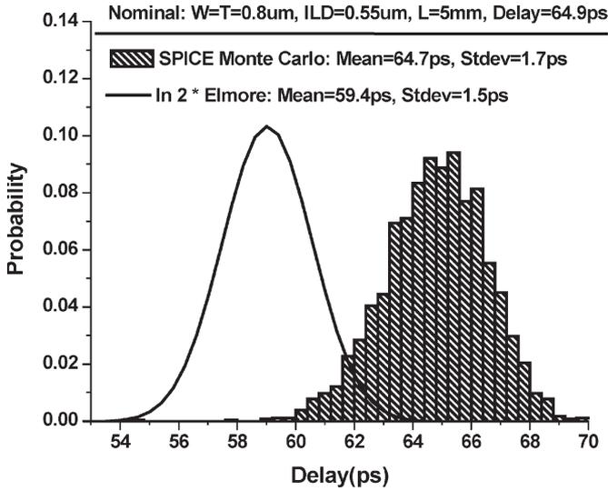
Fig. 5. Analytical delay distribution obtained using the statistical analysis of the scaled Elmore metric compared to Monte Carlo simulations. Nominal values (three-sigma tolerances) for metal width, thickness, and ILD height were  $0.8 \mu\text{m}$  ( $\pm 0.1 \mu\text{m}$ ),  $0.8 \mu\text{m}$  ( $\pm 0.1 \mu\text{m}$ ), and  $0.55 \mu\text{m}$  ( $\pm 0.05 \mu\text{m}$ ), respectively.
