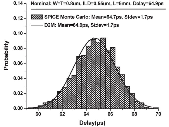
Fig. 6. Analytical delay distribution obtained using the statistical D2M metric compared to Monte Carlo simulations. Nominal values (three-sigma tolerances) for metal width, thickness, and ILD height were  $0.8 \mu\text{m}$  ( $\pm 0.1 \mu\text{m}$ ),  $0.8 \mu\text{m}$  ( $\pm 0.1 \mu\text{m}$ ), and  $0.55 \mu\text{m}$  ( $\pm 0.05 \mu\text{m}$ ), respectively.
