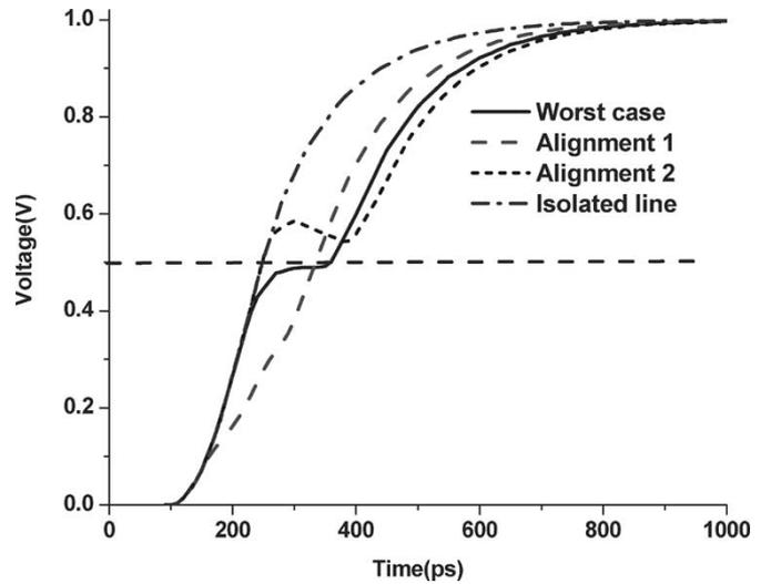
Fig. 15. Worst case alignment of noise peak that results in maximum delay degradation. Alignment 1 and 2 refer to the cases when noise peaks occur before and after this worst case alignment, respectively. These alignments have smaller impact on 50% switching time as compared to the worst case alignment.
