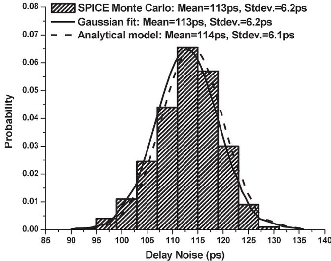
Fig. 16. Analytical coupling-induced dynamic-delay distribution compared to Monte Carlo simulations. The Gaussian-fit curve shows Gaussian fitting to the HSPICE mean and standard deviation. Nominal values (three-sigma tolerances) for metal width, thickness, and ILD height were  $0.65 \mu\text{m}$  (23%),  $0.5 \mu\text{m}$  (11%) and  $0.26 \mu\text{m}$  (11%), respectively. Nominal interwire spacing was  $0.4 \mu\text{m}$  and it was inversely correlated with width.
