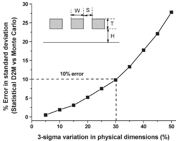
Fig. 19. Error in statistical D2M model as a function of percentage variation in physical dimensions.
