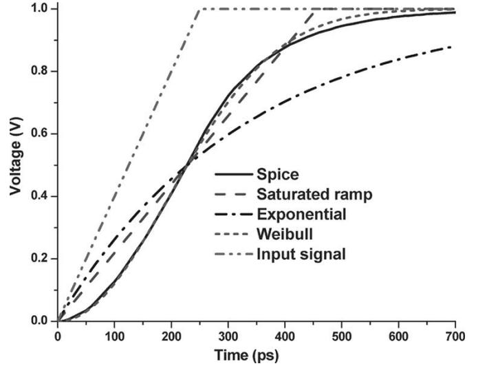
Fig. 14. Output waveform of an RC circuit under ramp input. The figure shows actual HSPICE results and various analytical approximations of the waveform.
