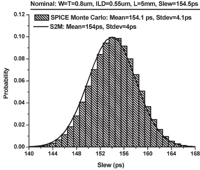
Fig. 7. Analytical slew distribution obtained using the statistical S2M metric compared to Monte Carlo simulations. Nominal values (three-sigma tolerances) for metal width, thickness, and ILD height were 0.8  $\mu$ m ( $\pm 0.1$   $\mu$ m), 0.8  $\mu$ m ( $\pm 0.1$   $\mu$ m), and 0.55  $\mu$ m ( $\pm 0.05$   $\mu$ m), respectively.
