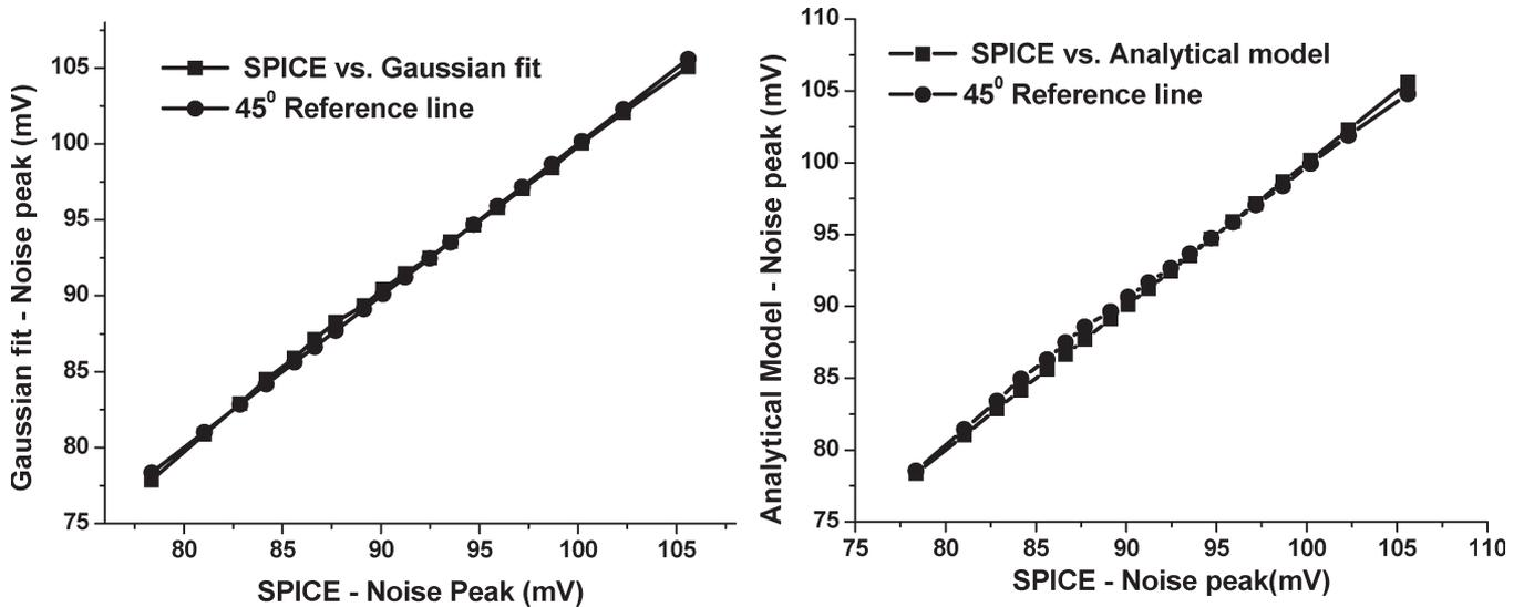
Fig. 11. q-q plots for noise peak: (Left) HSPICE results versus Gaussian distribution (with same mean and standard deviation as obtained from SPICE simulations) with 45° reference line. (Right) SPICE result versus the analytical model with 45° reference line. Nominal values (three-sigma tolerances) for metal width, thickness, and ILD height were 0.55 μm (14%), 0.44 μm (30%), and 0.3 μm (15%), respectively. Nominal interwire spacing was 0.4 μm and it was inversely correlated with width.
