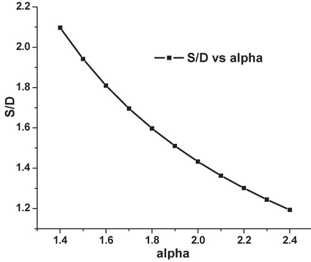
Fig. 13. Slew/Delay ( $S/D$ ) as a function of Weibull parameter  $\alpha$ . A second-order-polynomial fitting is used to express  $S/D$  in terms of  $\alpha$ .
