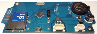
Figure 8: The datalogger PCB. Our system supports complex subcircuits such as microcontrollers application circuits and analog power generators such as the current-limited supercapacitor backup.
