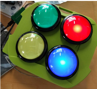
Figure 7: The Simon PCB with connected buttons. Our system is able to generate the 5v to 12v boost converter subcircuit to drive the LEDs in the dome buttons.
