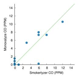
Figure 6: A comparison of Smokerlyzer CO measurements and Monoxalyze CO measurements. taken from a trial of 13 participants at a smoking cessation clinic. One of 13 trials failed to collect data, so 12 data points are plotted. The diagonal line shows the ideal correlation between the Smokerlyzer and Monoxalyze. This shows that Monoxalyze is reasonably accurate compared to the Smokerlyzer, which is considered the gold standard for smoking cessation determination.
