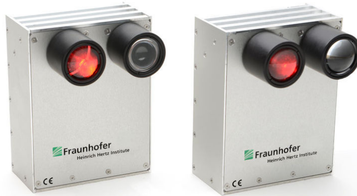
Figure 2.7: High speed VLC transceiver. Heinrich Hertz Institute developed a VLC transceiver operates at 500 Mbps at 4 m or 120 Mbps at 20m. It uses OFDM modulation to achieve high data rate and features bidirectional communication [35].
