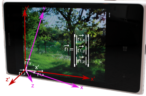
Figure 6.3: Receiver orientation. The vectors x' , y' , and z' are defined as shown in the picture. The projection of the unit vectors \hat{x}' , \hat{y}' , and \hat{z}' onto the x , y , and z axes in the transmitters' frame of reference gives the elements of the rotation matrix \mathbf{R} .
